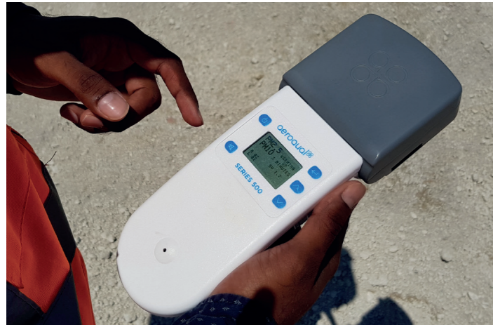
Portable dust monitors are used regularly throughout the Bay Link site.
