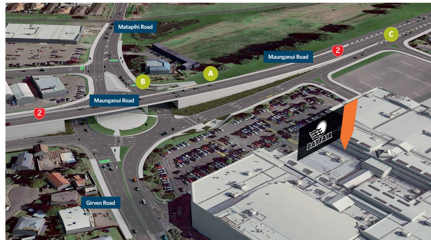
An artist's impression of what the Bay Link project near Bayfair will look like. Current work in the Bayfair roundabout area is focusing on ground improvement works for the new underpass (A), constructing the approaches to the new Bayfair roundabout (B) and the new road and footpaths on Maunganui Road near Bayfair (C).
