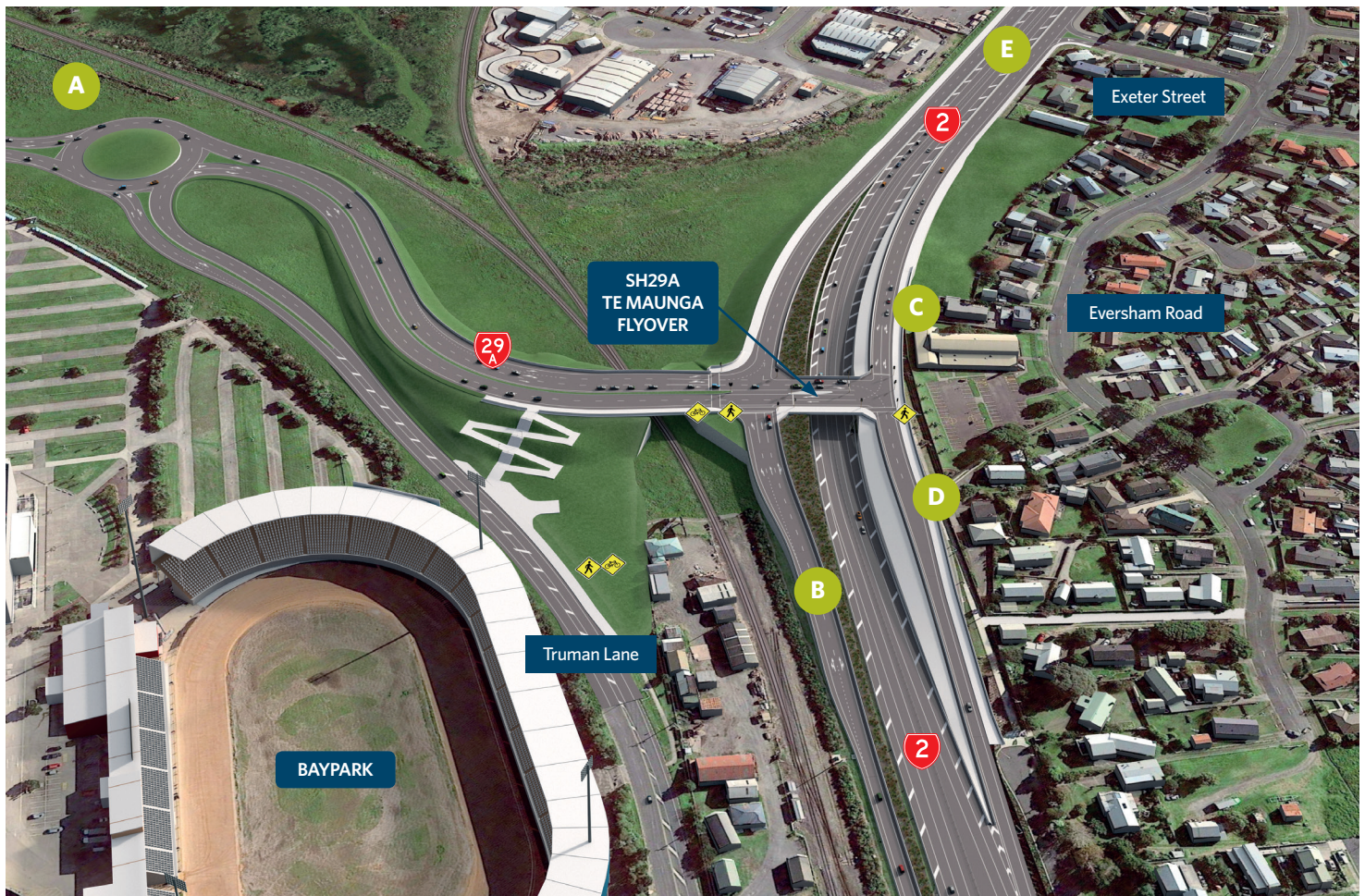
An artist's impression of what the Bay Link project near Baypark will look like. Current work in this area is focusing on the new Baypark roundabout (A) and stone column ground improvement works (B, C and D).
