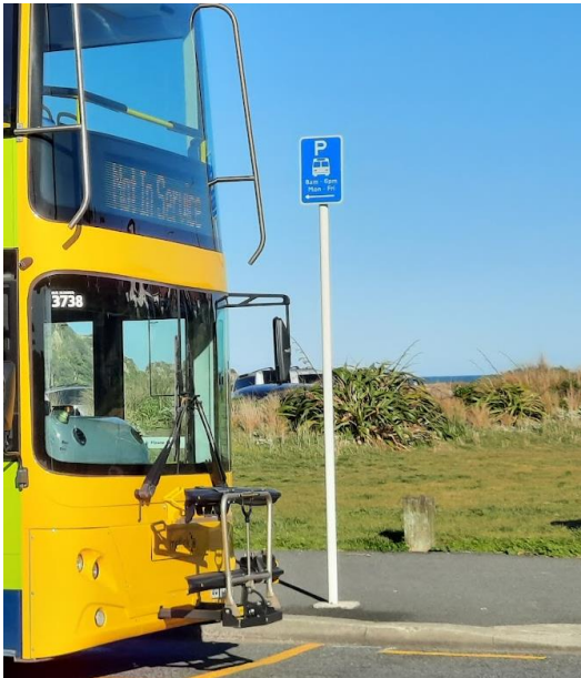
Figure 21: Example of a bus layover space with the recommended R6-53 bus parking sign (Source: Lorelei Schmitt).
