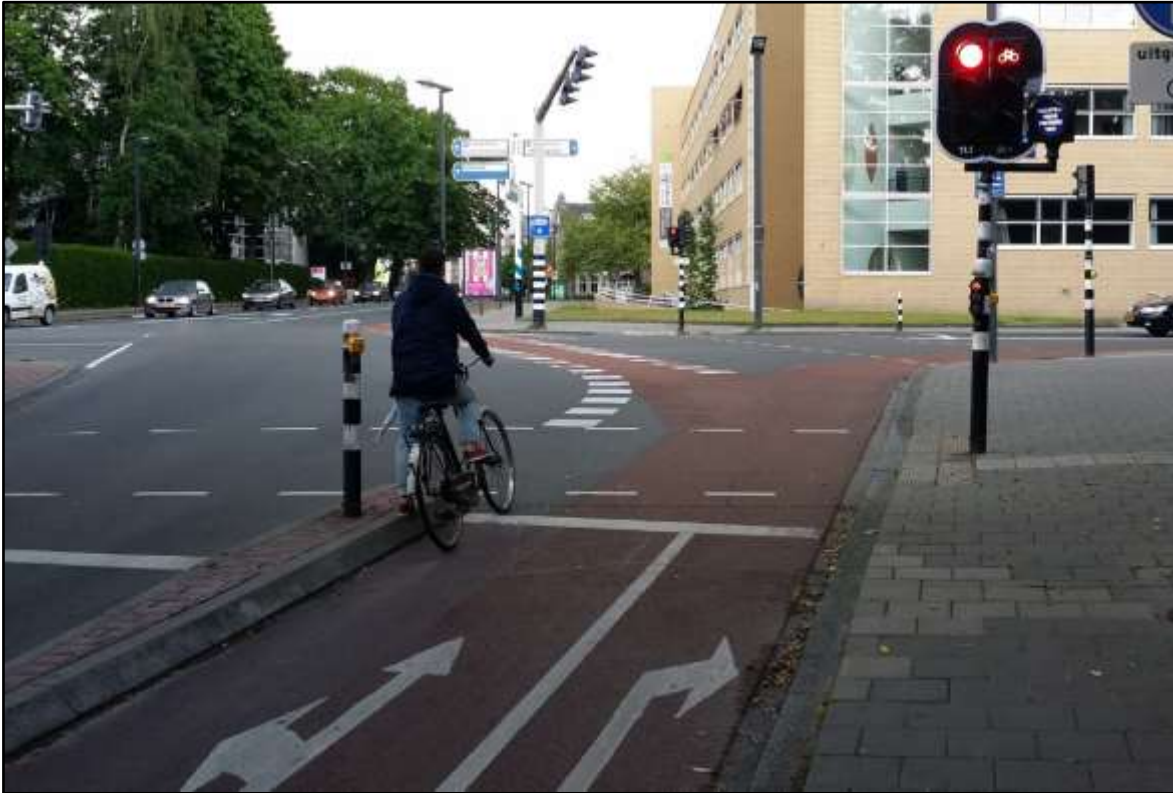
Figure 6-6: Sign next to the signals says “right turn free for cyclists”, Enschede, Netherlands
