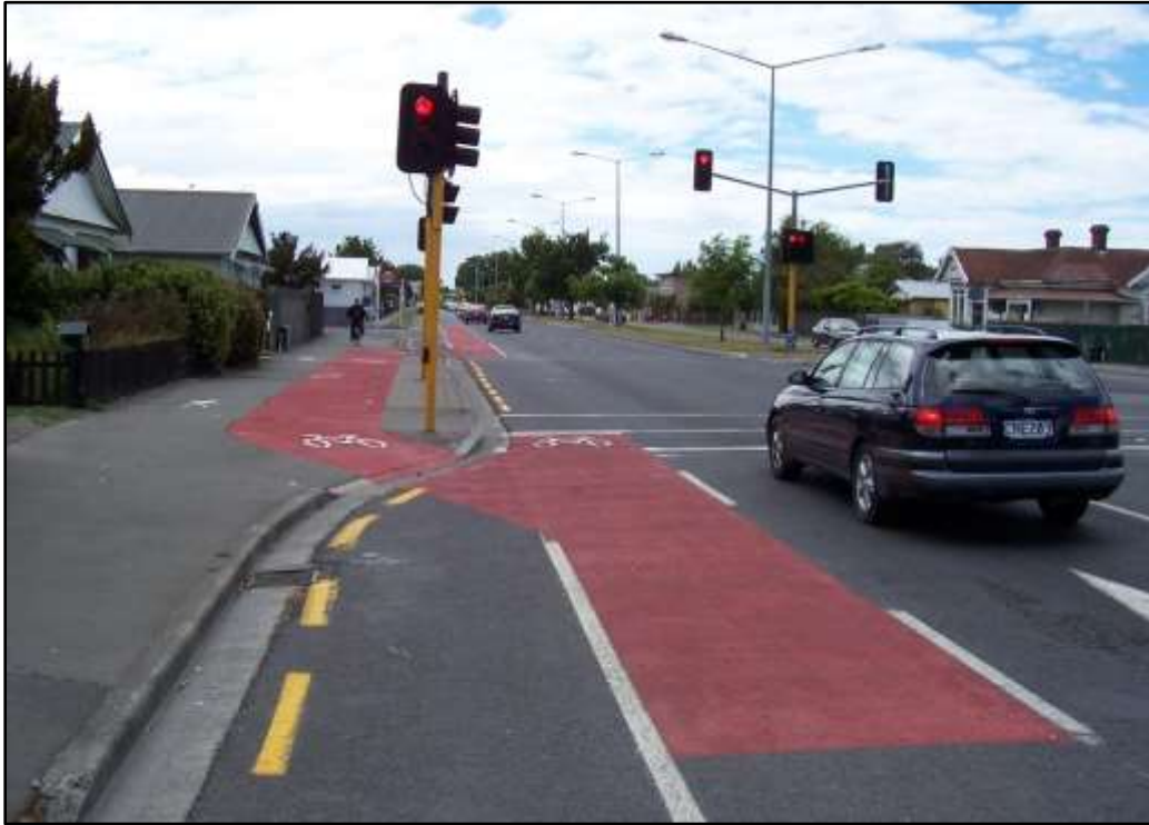
Figure 6-2: Example of a “top of T” cycle bypass, Buckleys/Russell intersection, Christchurch
