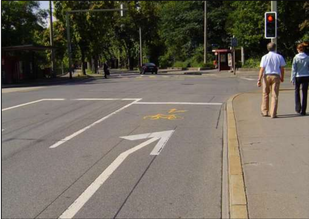
Figure 3-6: Cycle markings allow cyclists to go straight from a right-turn lane, Winterthur, Switzerland
