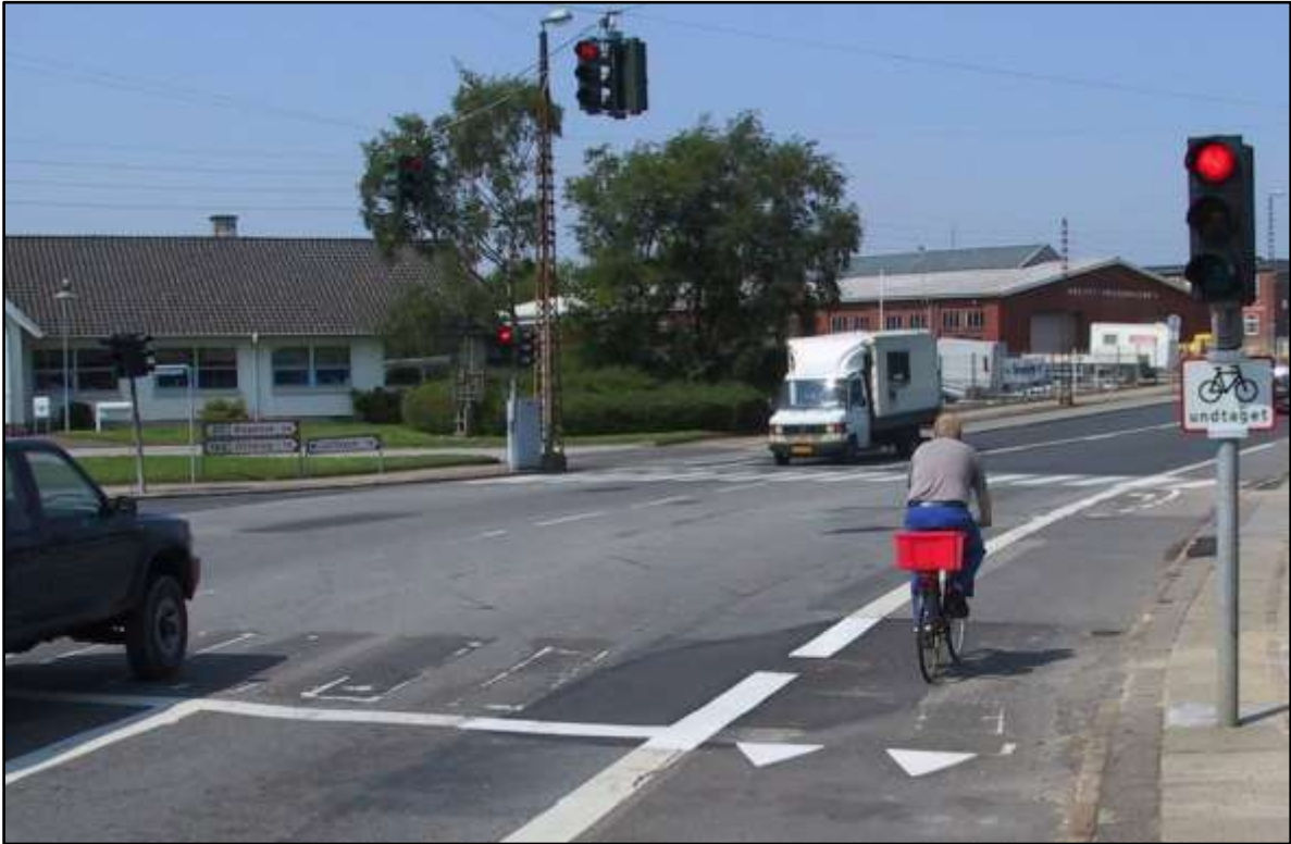
Figure 6-7: Cyclists allowed to ride through top of the T, Odense, Denmark (“undtaget” = “except”)
