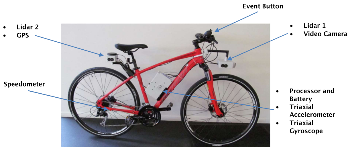
Figure 8.1. A detailed illustration of the instrumented bike technology.
