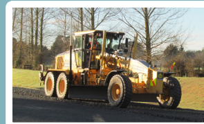
Top: An articulated dump truck. Bottom left: A grader shaping pavement material. Bottom right: A scraper which is used to move dirt over short distances.
