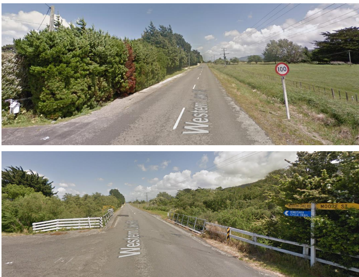
Figure 3.1: Existing location of speed limit threshold (top) and new location of speed limit threshold (bottom) looking south (Source: Google Maps)
