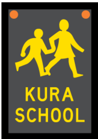
Figure 2.3: W19-2.1 Warning – symbol illuminated when activated (Kura School) — Permanent warning
