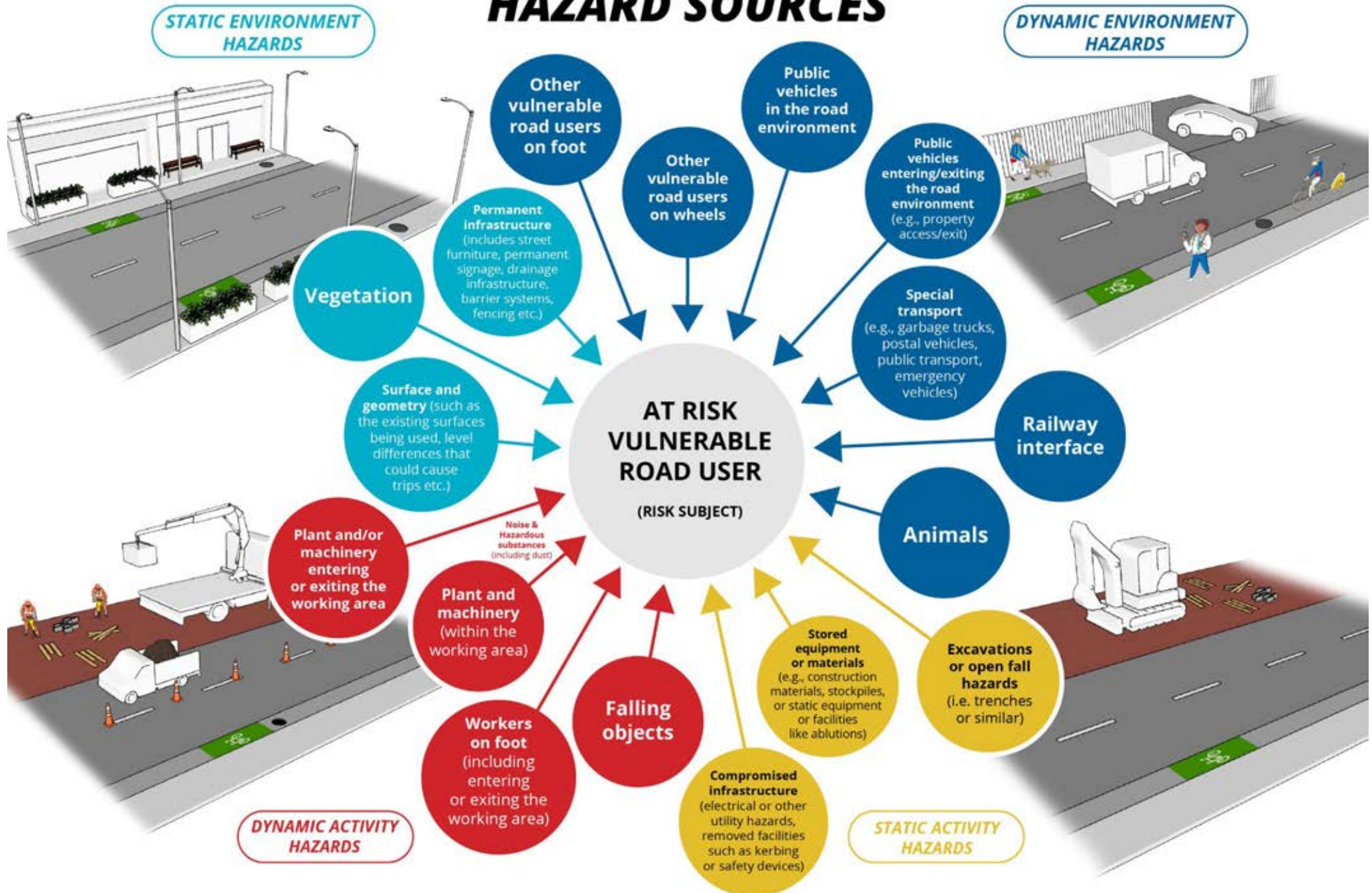
Figure 5 - Hazard sources for Vulnerable Road Users in TTM environments
