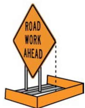
When not installed properly, all signs can be hazardous for the public. If signs are in place for some time, consider a detectable edge for cane users safety. Image Credit Ixxv: Minnesota Department of Transportation.
