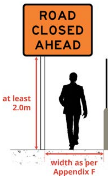
Figure 23 – Pedestrian or cycling box dimension requirements
