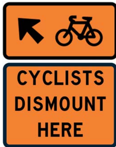
Figure 21 - This sign combination uses a W5-8.12 cyclist directional sign, with a custom sign under W8-8 from the Traffic Control Devices Rule 2004.
