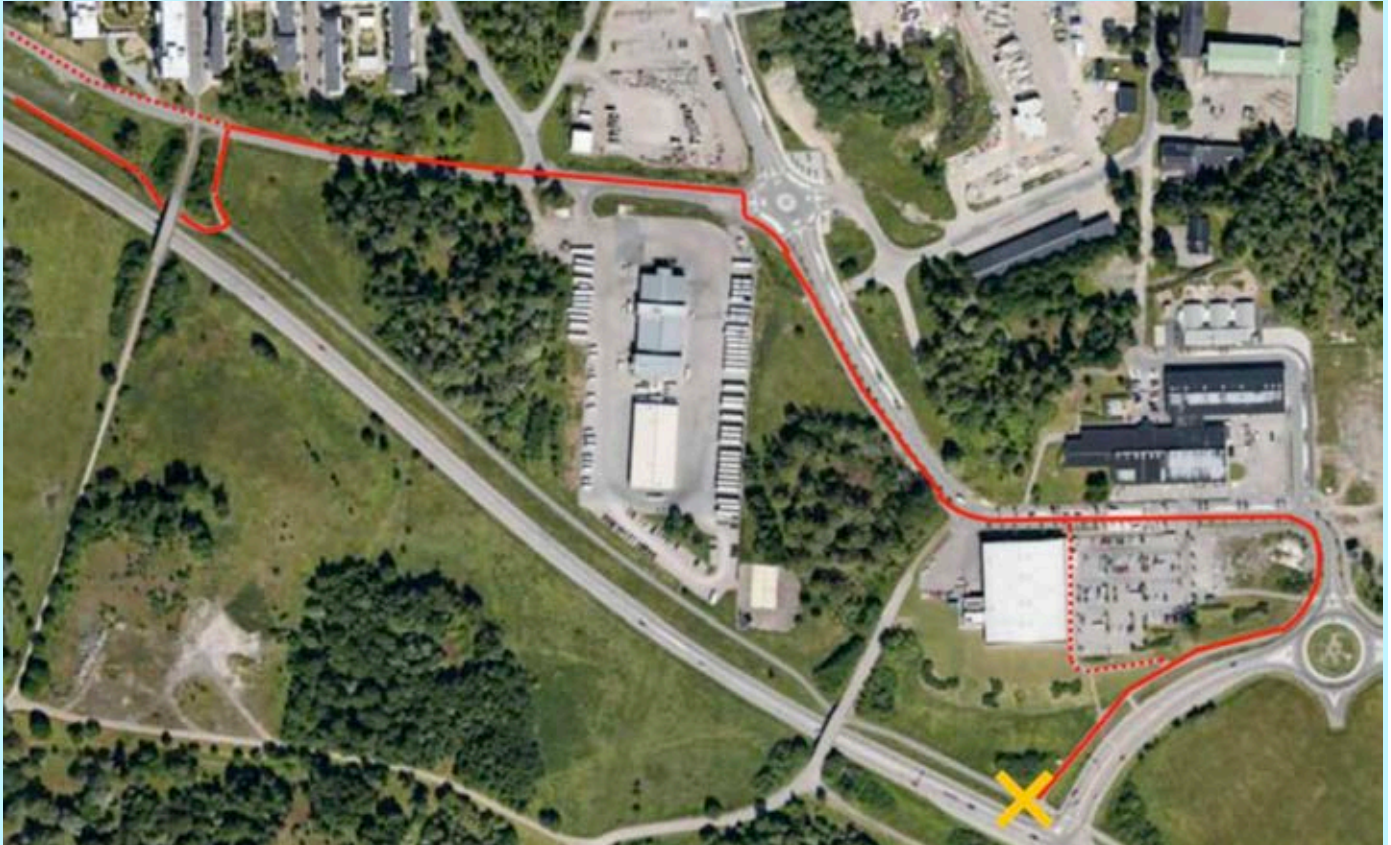
Rerouting of cycle traffic when the cycle path is closed (yellow cross) due to roadworks. The solid red line shows the route the cyclists are directed to, while the dotted lines show their chosen route. Image Credit lii: www.eniro.se
