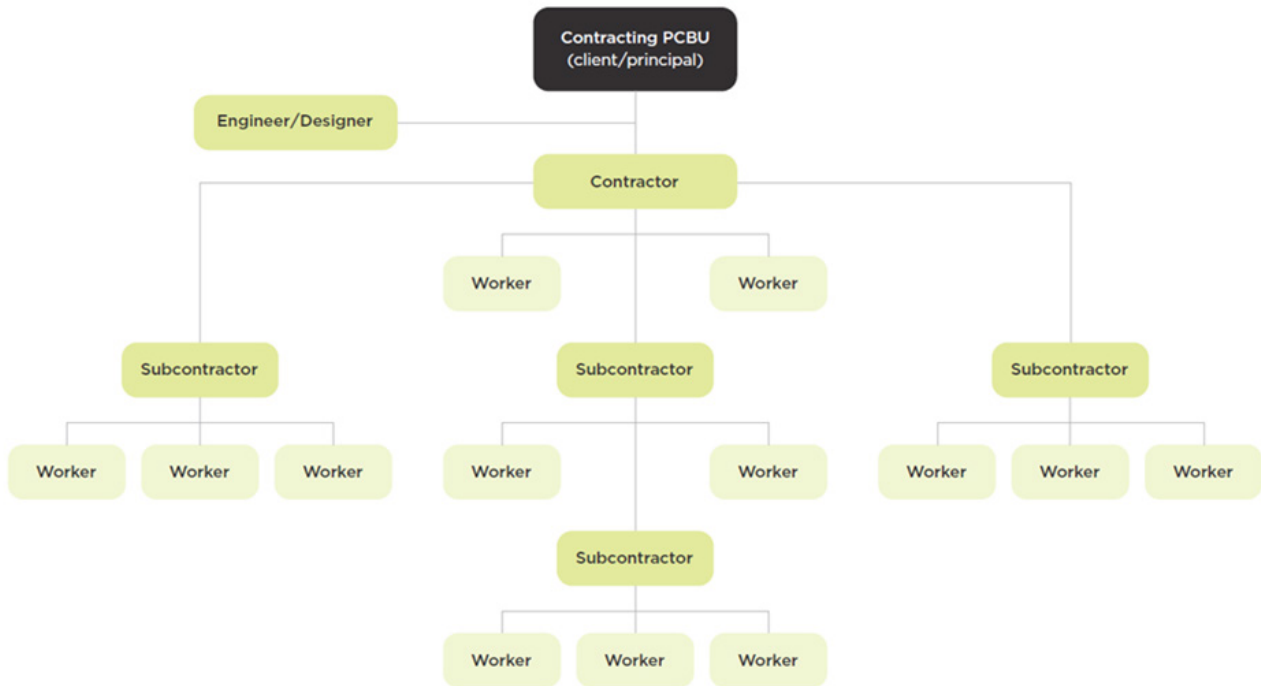
Figure 3: Example of a contracting chain. Image credit: WorkSafe
