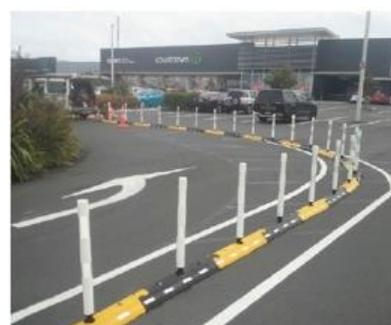
**Figure 19: spacing of posts on a continuous low separator**
