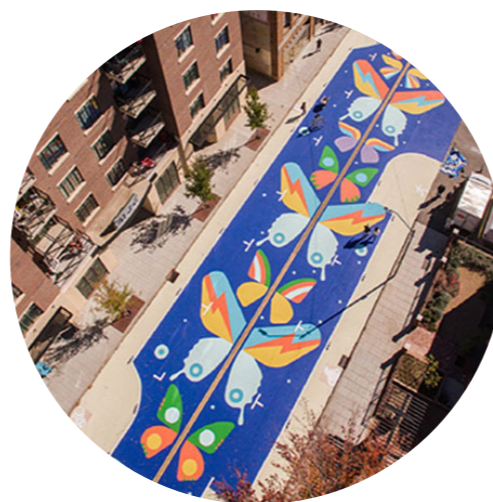
Roadway art, widened footpaths and a barrier-protected multiuse path installed in Asheville, North Carolina, helped to reduce speeds on Coxe Avenue by 28.3%, and reduced incidents of speeding from 66% to 21%. Source: Asphalt Art Guide, Bloomberg Associates
