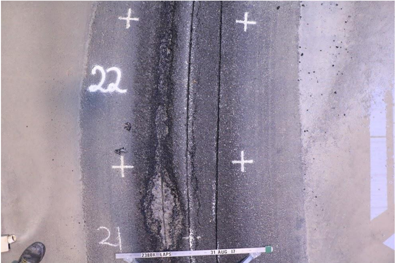
Figure 40 100,000 Laps of Wet Running after saw-cutting surface
