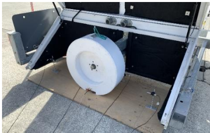
Figure 3. Tyre shaped sound source mounted to CPX trailer.
