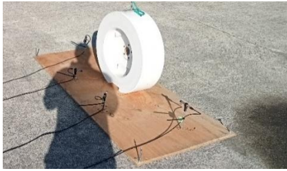
Figure 2. Tyre shaped sound source on reflective plane.
