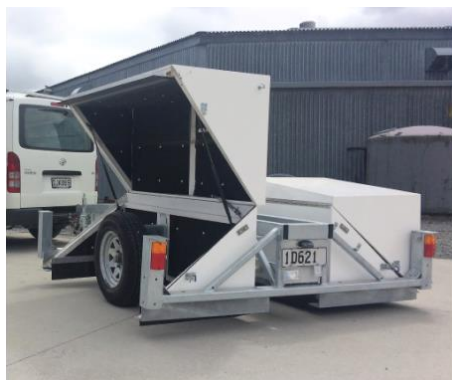
Figure 1. Waka Kotahi trailer based CPX system.
