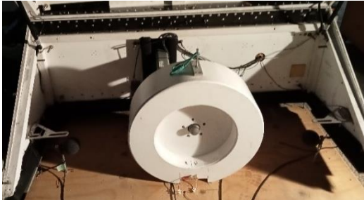
Figure 8. Absorption removed from enclosure (tyre shaped source).
