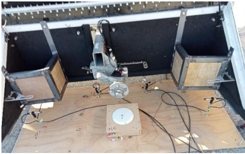
Figure 7. Reflective boxes in enclosure (cuboid shaped source).
