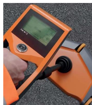
Figure 2. Measurement of thickness by magnetic induction
