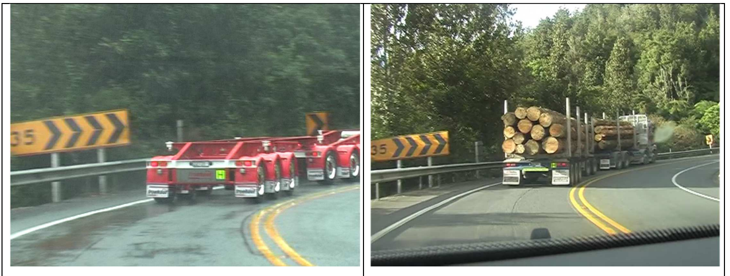
Figure 5. Traversing a 35 km/h advisory speed curve – pro-forma B-train compared to pro-forma log truck.
