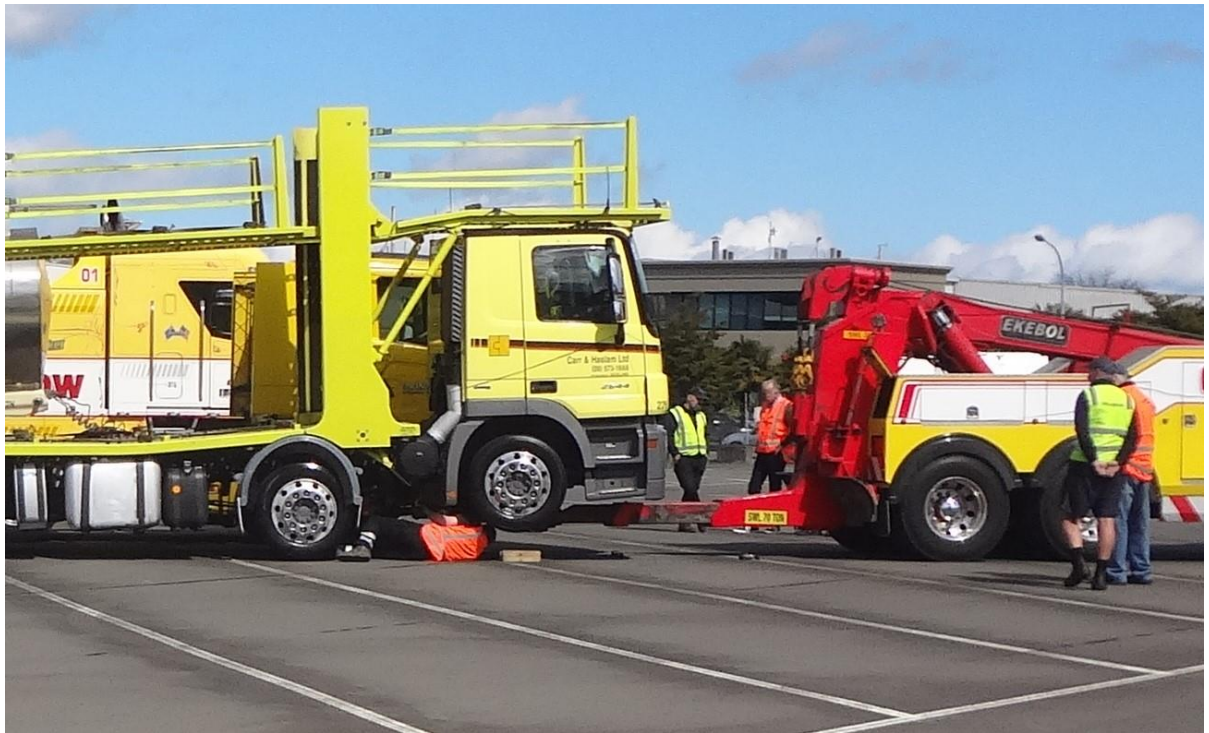
Figure 6. Towing connection to the front axle of the towed vehicle.
