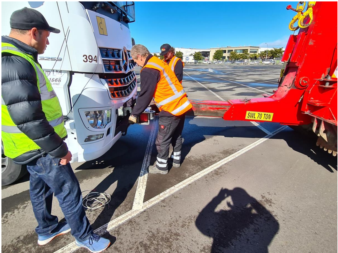
Figure 5. Connecting the tow truck to the 23m truck and trailer.
