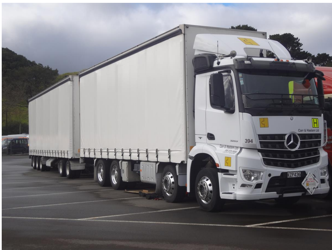
Figure 1. Carr & Haslam 23m linehaul truck and trailer combination.
