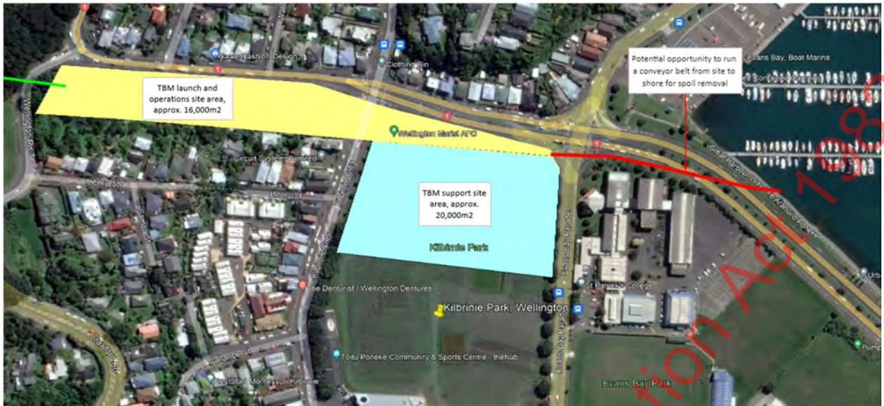
Figure 10. TBM work area (South end at Kilbirnie)
