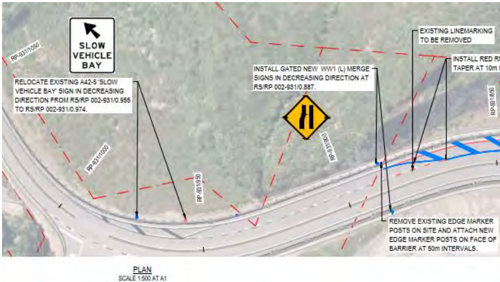
Figure 10: Short Slow Vehicle Bay with ineffective passing length.
