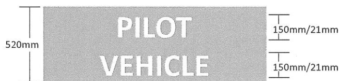
Figure 4—Warning sign for pilot vehicle (Ref. 5.7(16))
