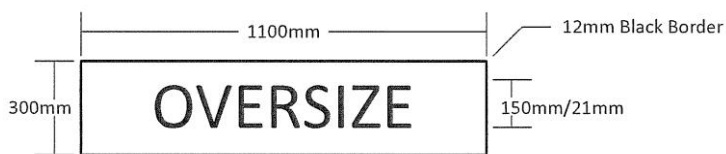
Figure 3—Dimensions of ‘OVERSIZE’ sign for overdimension vehicles (Ref. 5.4(13)(a))
