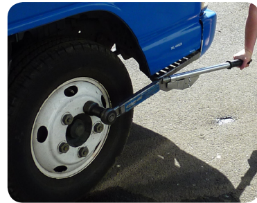
Torque wrench in use
