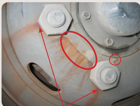
Rust marks indicating loose wheel nuts and cracked wheel disc
