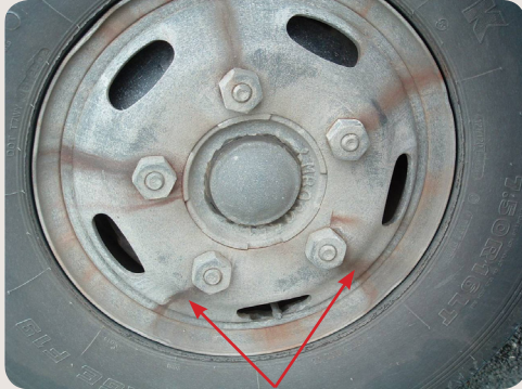
Rust marks around a wheel nut is a sure sign that the nut is loose
