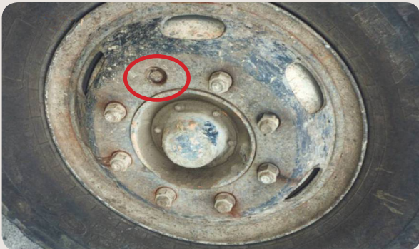
A broken wheel stud - usually caused by over-tightening
