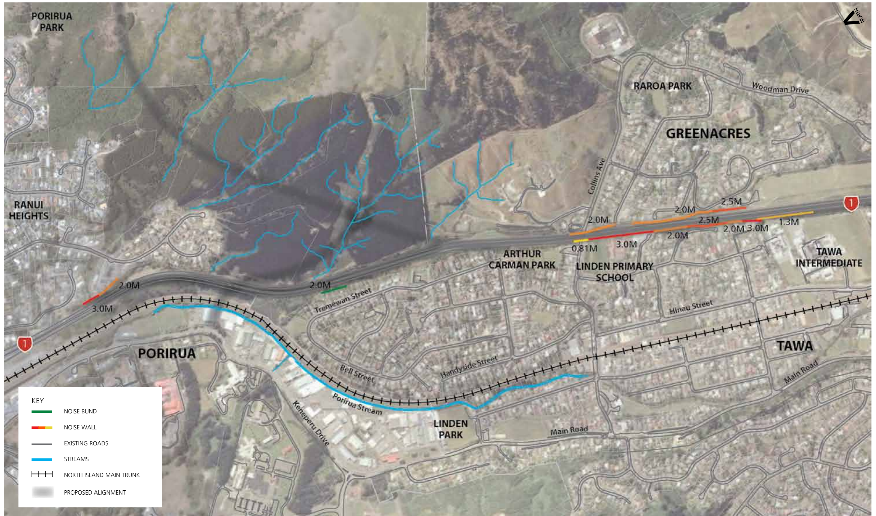
Figure 5.83: Proposed location and height of noise barriers
