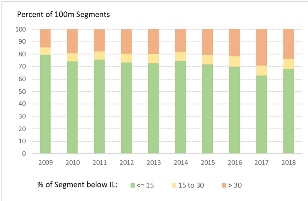
Figure 20: Breakdown of % of segment length ESC below IL
