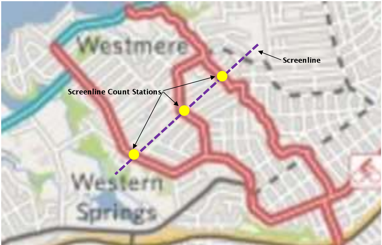
Figure 4: Screenline Example (Auckland)
