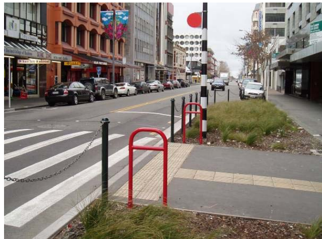
Figure 1: Hereford Street site, Christchurch Note detection units, kerb build out and barriers to channel pedestrians. Source: MWH 2008
