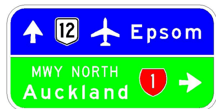
FIGURE 7.1: AD - 1 ADVANCE DIRECTION SIGN
