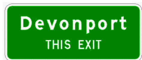
FIGURE 4.1: AN MI - 6 FORMAT SIGN INDICATING THAT THE NEXT EXIT PROVIDES ACCESS TO AN IMPORTANT PLACE NOT ON THE EXPRESSWAY/MOTORWAY ROUTE
