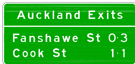
FIGURE: 4.4: AN MI - 7 FORMAT SUPPLEMENTARY DESTINATION SIGN INDICATING MULTIPLE EXITS TO A PLACE OR IMPORTANT FACILITY AND DISTANCES TO THE EXITS
