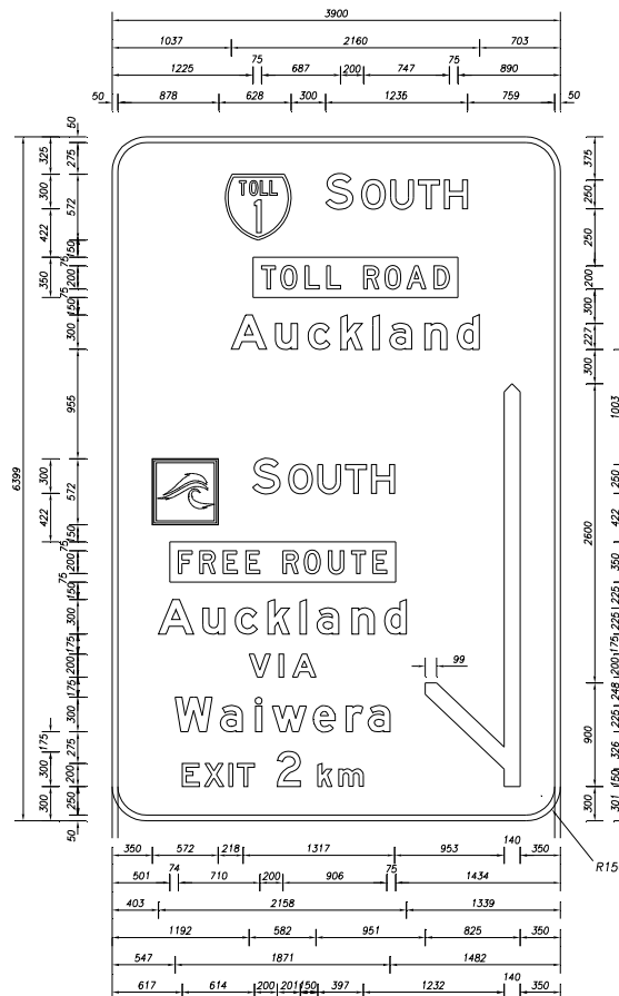
MI - 1 DIAGRAMMATIC ADVANCE EXIT SIGN WITH 'TOLL ROAD' AND 'FREE ROUTE' PANELS
