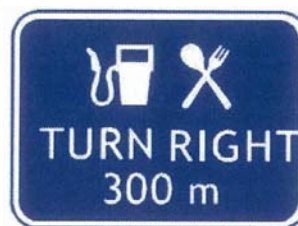
Figure 5.21 Advance sign indicating services on a side road
