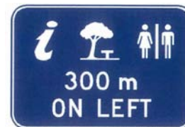
Figure 5.17 Advance sign indicating rest area adjacent to road
