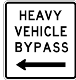
Figure 4.25 Heavy vehicle bypass intersection position sign
