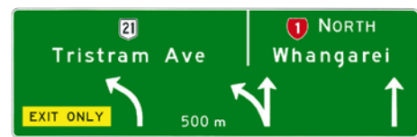
Figure 4.19 Layout for overhead advance exit sign with an exit only panel combined with standard lane designations
