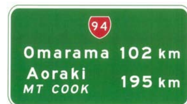
Figure A-2 Confirmation direction sign (longer secondary name than primary name) with distance centred between the two names
