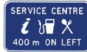
Figure 5.3 Commercial services advance sign
