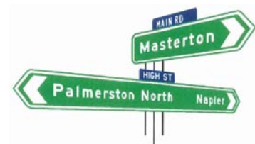
Figure 4.24 Side road signed above through route, with street name plates
