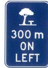
Figure 5.8 Advance sign rest area adjacent to road
