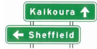
Figure 4.23 Offset intersection direction signs
