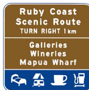
Figure 6.4 Combined advance tourist facility and services sign
