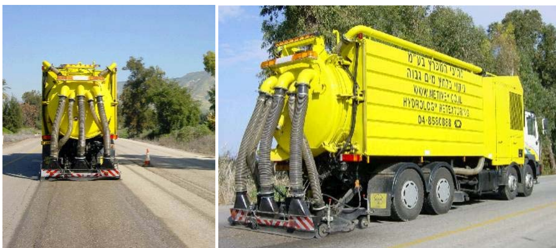
Figure 11: General view of a water blasting truck that works in Israel
