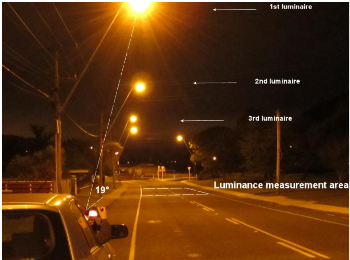
Figure 21 Photograph / Luminance measurement position showing the camera 1.25m above the road surface 0, the 19° elevation to the first luminaire, and the measurement area between the second and third luminaires.
