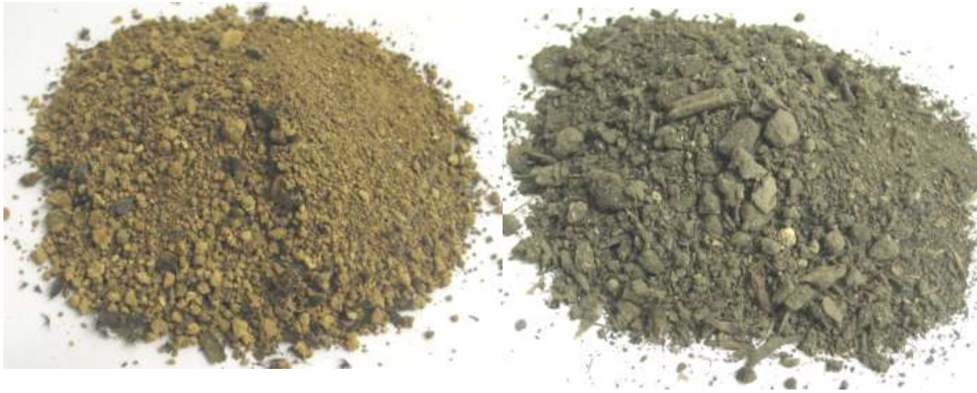
Figure 6-8 <9mm fraction of RDS from 'Sweeping-SH22' AMA-5 (left) and 'Catch pit-SH18' AMA-6 (right)
