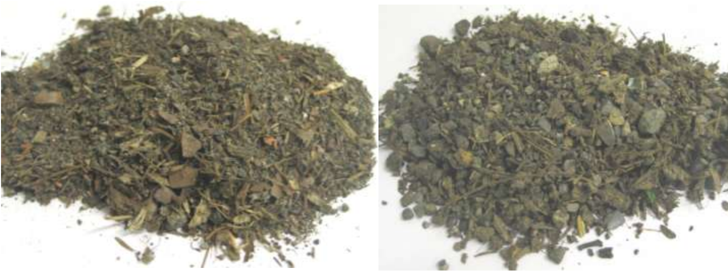
Figure 6-7 <9mm fraction of RDS from 'Sweeping-CMJ' AMA-3 (left) and 'Sweeping-Oteha' AMA-4 (right)
