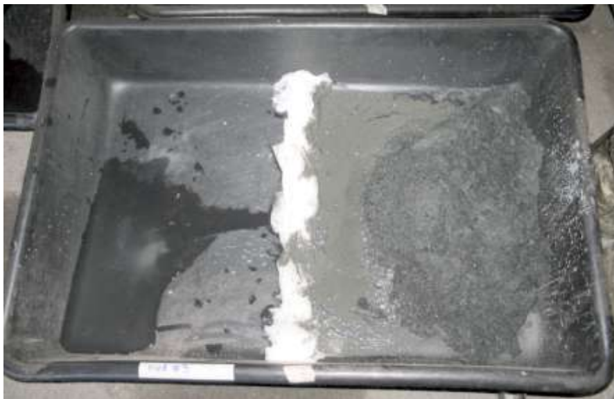
Figure 0-5 - Dewatering RDS sediment (AMA-2, 'Pond-causeway')
