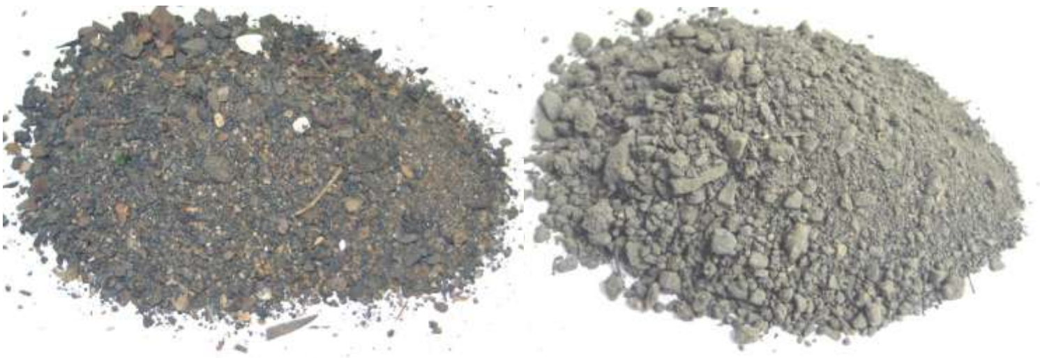
Figure 6-6 <9mm fraction of RDS from 'Pond-CMJ' AMA-1 (left) and 'Pond-causeway' AMA-2 (right)
