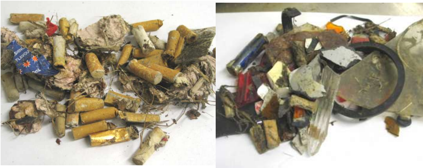
Figure 6-19 Litter in >9mm RDS fraction from 'Sweeping-CMJ' AMA-3 (left) and 'Sweeping-Oteha' AMA-4 (right)
