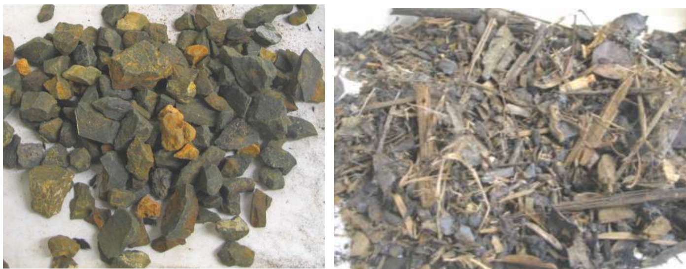
Figure 6-15 >9mm fraction of RDS from 'Sweeping-SH22' AMA-5 (left) and 'Catch pit-SH18' AMA-6 (right)
