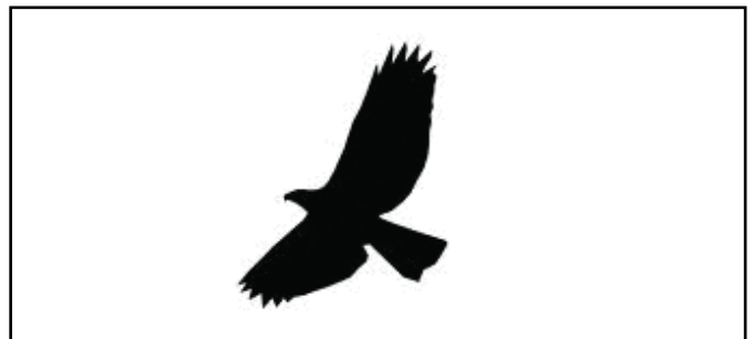
Figure 4.15 Bird decals can be applied to transparent panels to discourage bird strike
