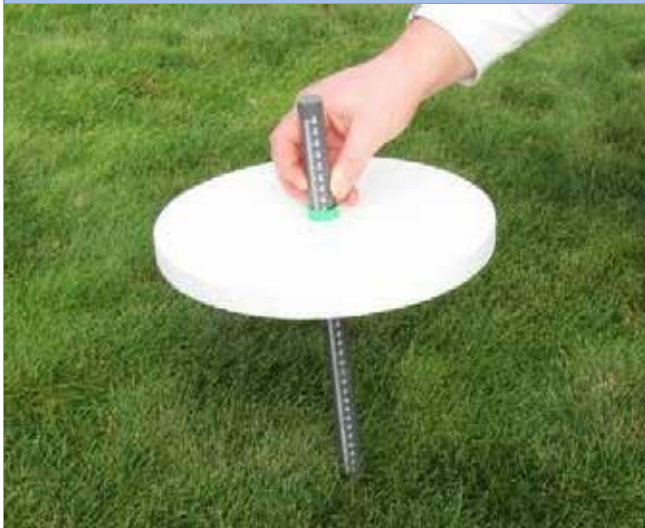
Example of rising disc meter for measuring grass height
