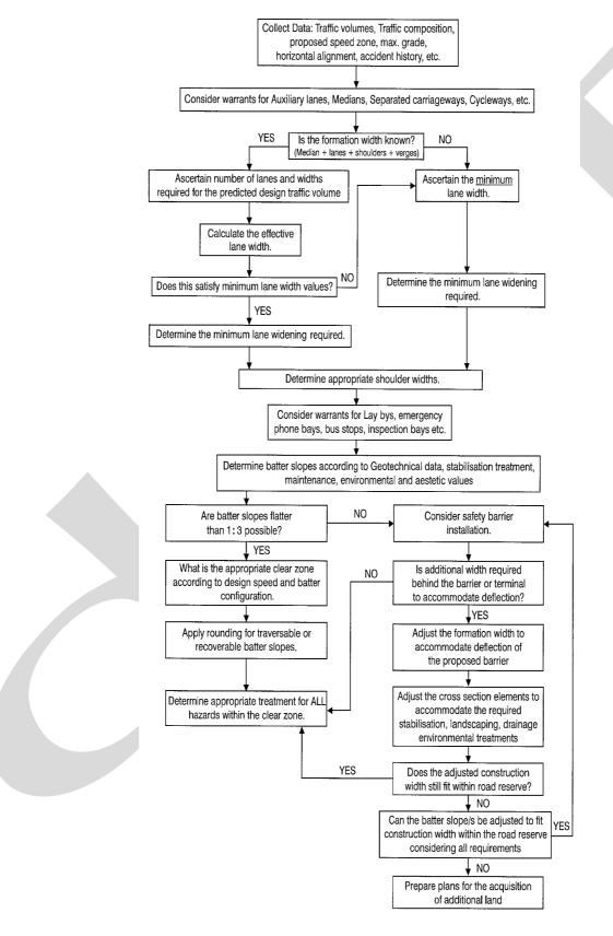
Figure 6.2: Cross Section Determination Flow Chart
