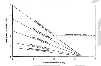
Figure 6.5: Lateral Forces on Cyclists Caused by Heavy Vehicles
