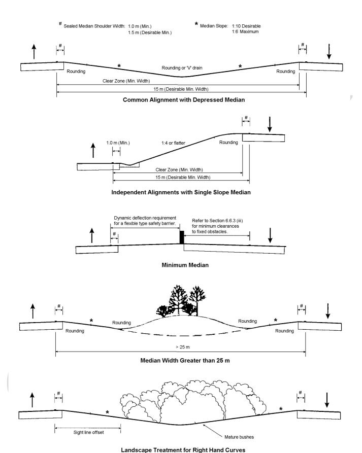
Figure 6.19: Typical Rural Median Cross Section Details
