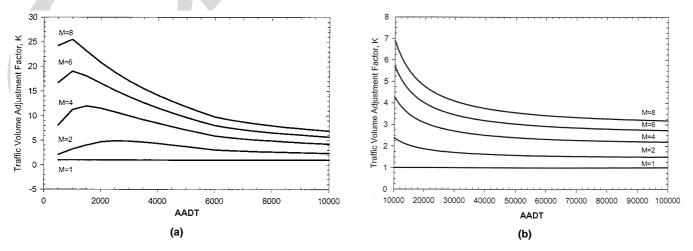
Figure 6.15: Traffic Volume Adjustment Factor, K, for Dual Carriageway Roads
