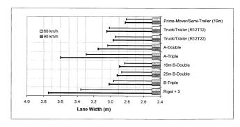
A clearance component is not included in these estimated vehicle path lane widths. Typically, 0.5 m needs to be added to give a lane width sufficient for efficient traffic operations.
