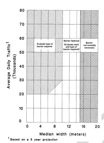
Figure 6.17: State Highway Median Barrier Warrant
