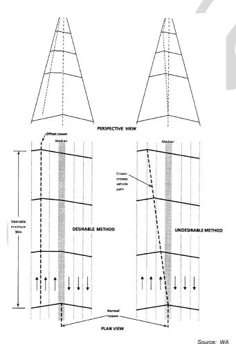
Figure 6.8: Development of a Longitudinal Crown on a One-way Road Carriageway
