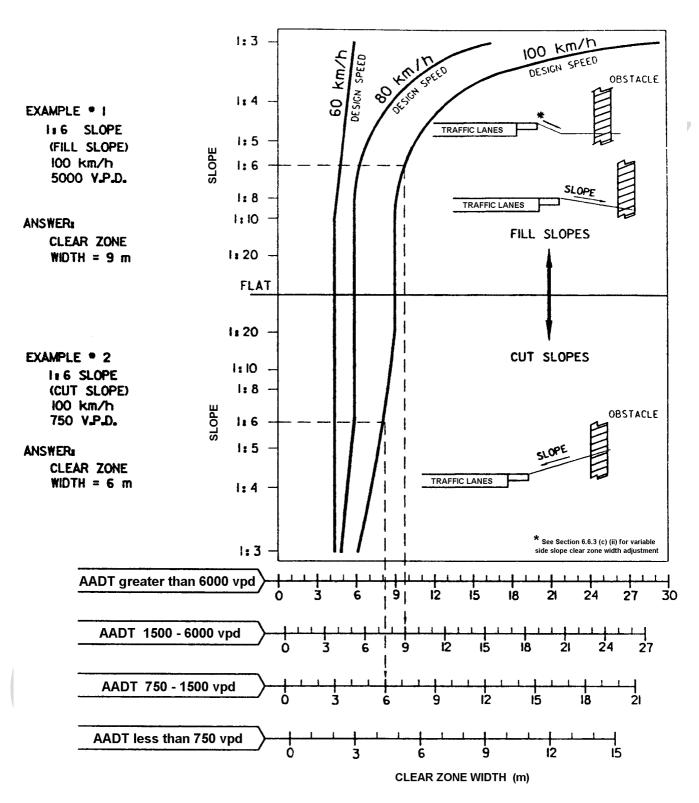
Figure 6.12: Clear Zone Width Required on a Straight Level Section of Road
