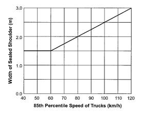
Figure 6.6: Recommended Sealed Shoulder Widths to Safely Accommodate Cyclists
