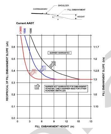
Figure 6.16: State Highway Fill Embankment Safety Barrier Warrant
