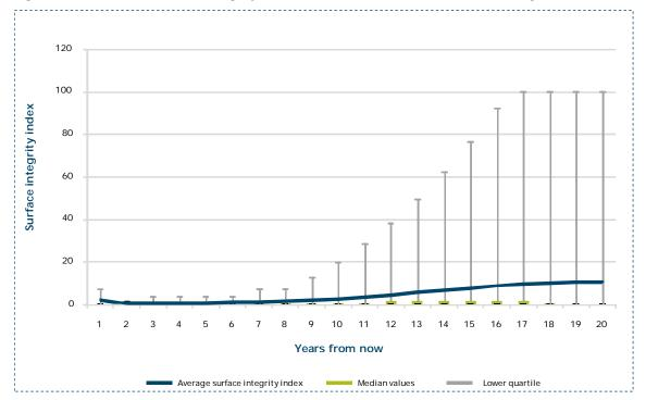
Figure 9.10 Modelled surface integrity index condition trend for constrained budget level
