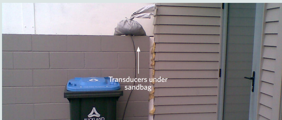
FIGURE 30: INCORRECT TRANSDUCER LOCATION
