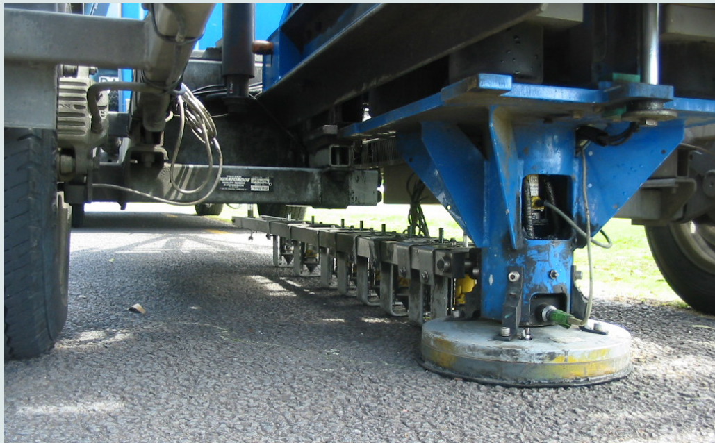
FIGURE 22: FALLING WEIGHT DEFLECTOMETER
