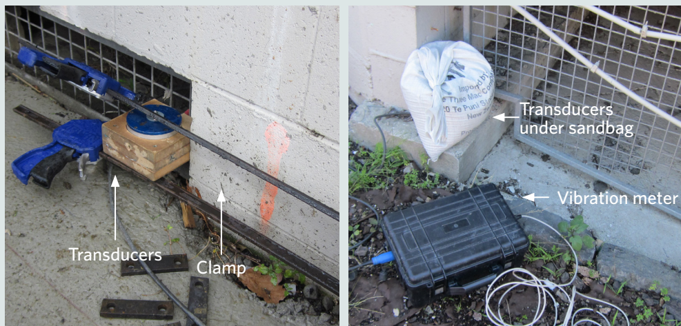
FIGURE 30: INCORRECT TRANSDUCER LOCATION
