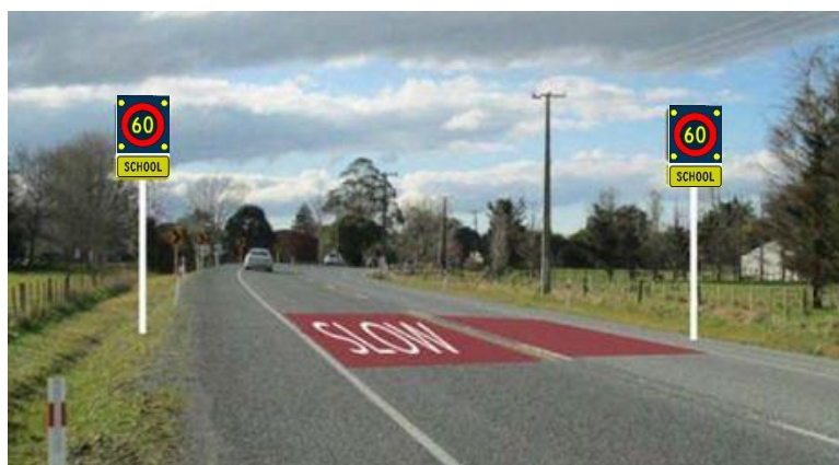
Figure 13. Variable speed limit configuration soon to be trialled by Auckland Transport
