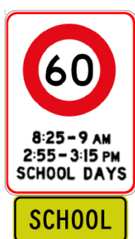
Figure 11 Static variable speed limit signs installed on side roads within variable speed limit area.
