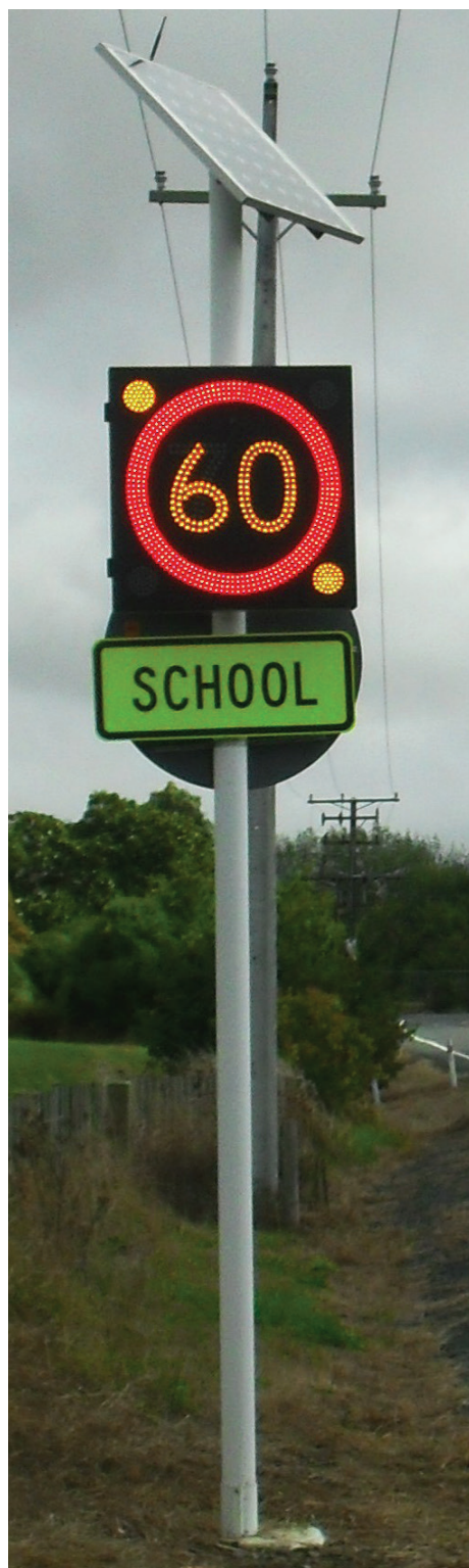
60km/h variable speed limit school trial sign
