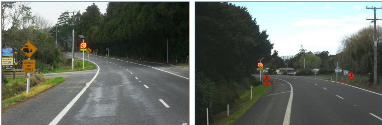
Figure 25 (i&ii) 40km/h LED Mandatory Speed Sign Installed - Left: Northbound, Right: Southbound
