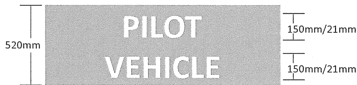
Figure 7.6—Warning sign for pilot vehicle (Ref. 6.42(3), and 6.43(3))
