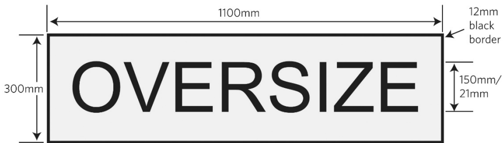
Figure 7.5—Dimensions of “OVERSIZE” sign for overdimension vehicles (Ref. 6.18(2))
