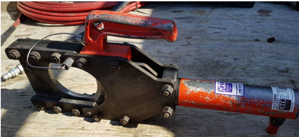
Image 2: An example of a remotely operated hydraulic wire rope cutter.
