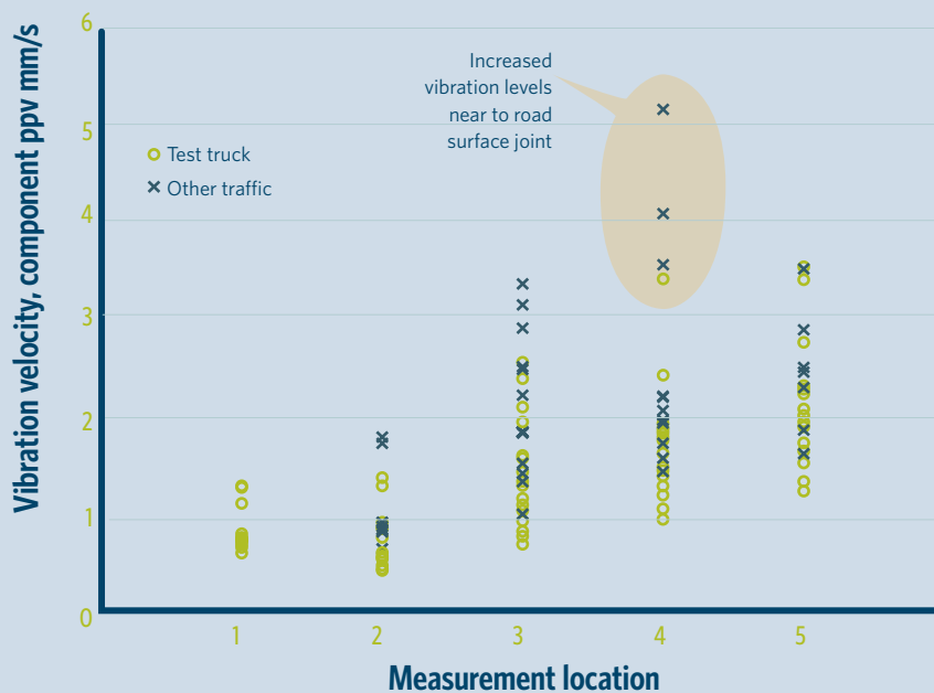
FIGURE 3.11 | Measured vibration levels at 5m from the road edge
