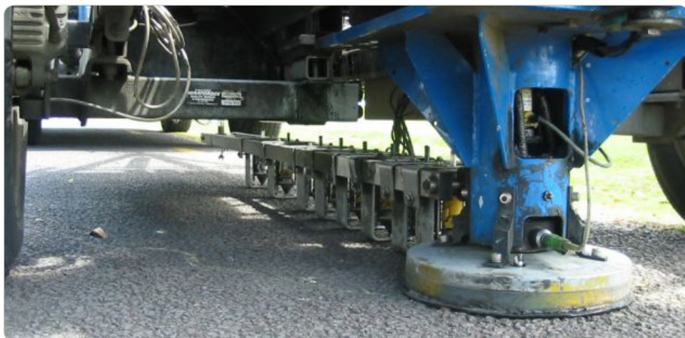
FIGURE 3.1 Falling weight deflectometer
