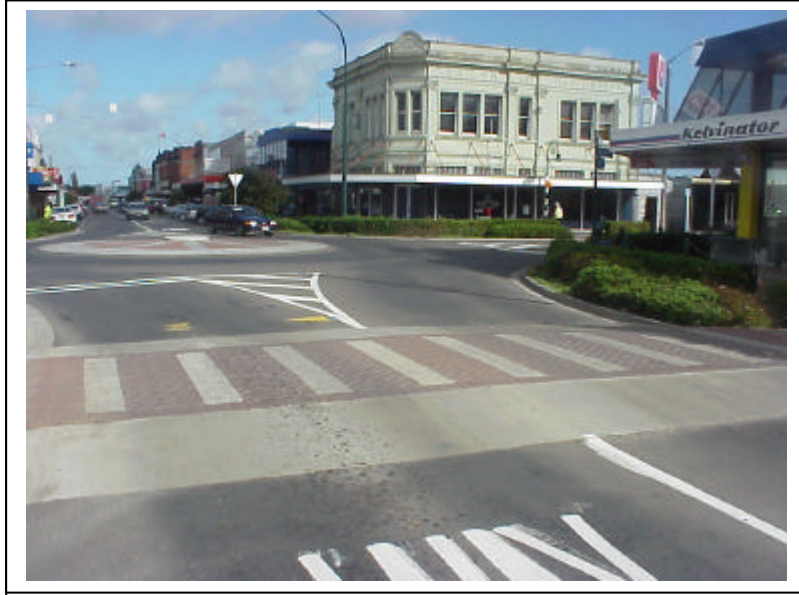
Photograph 11 : Pedestrian crossing/platform on approach to small roundabout.
