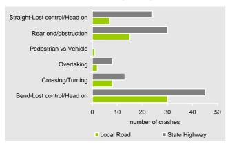
A significant number of crashes, especially on the state highways, were rear end obstruction and straight – lost control/heads-on types.
