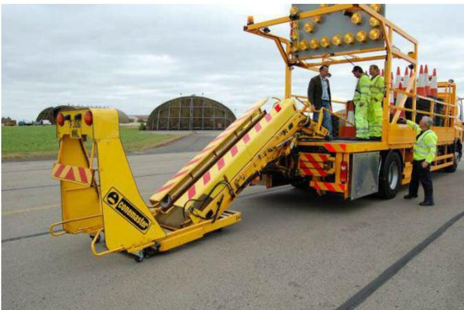
A less cumbersome Dutch semi-automatic system, the Verheij 4012, still requires a worker on the back of the truck (Figure 2.31).
