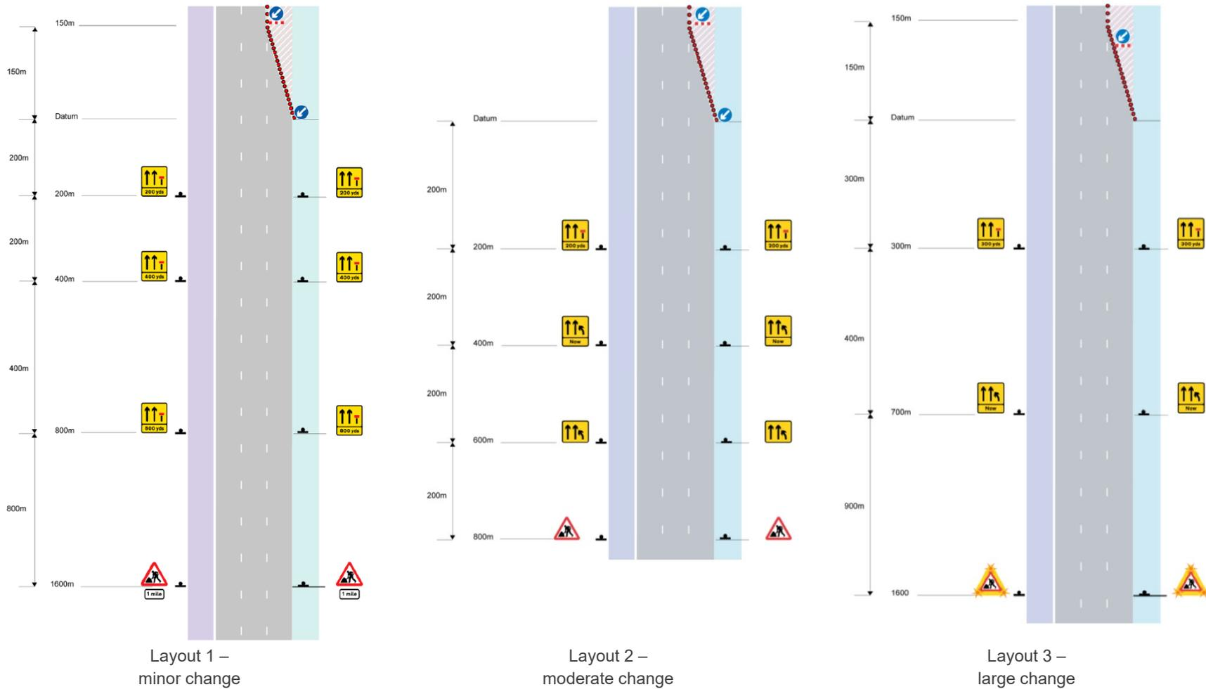
Figure 2.16 Two alternative lane closure layouts trialed (reprinted from Wood et al., 2011, p. 14)
