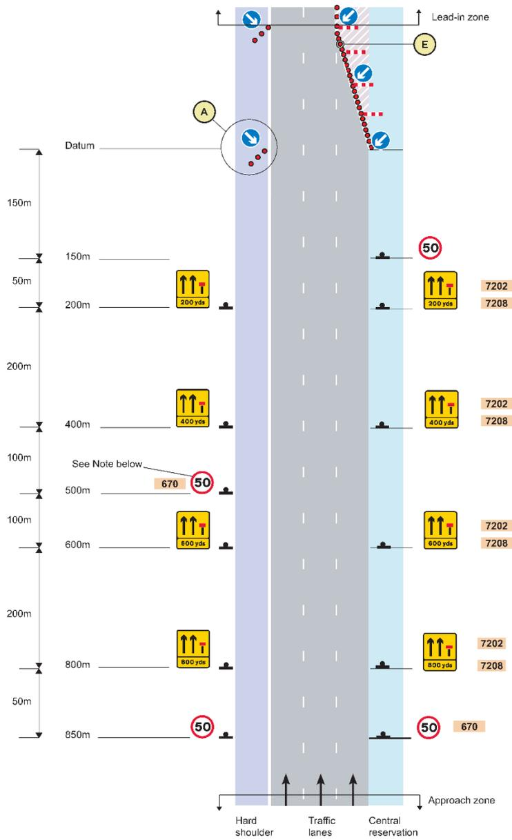
Figure 2.15 Alternative layouts for single-lane closures on dual carriageways (reprinted from Wood et al., 2011, pp. 7–9)
