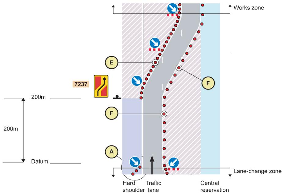
To install the ‘facing wall of cones’, workers must enter the only remaining open lane in the face of oncoming traffic, utilising what gaps they can find in the stream – a risky activity. If the work zone is left with the wall incomplete due to the low traffic window of opportunity passing, risk to road users is heightened due to the incomplete lead-in zone.
