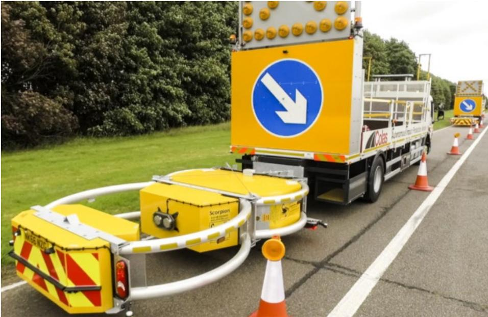
The autonomous IPV possesses a ‘Leader/Follower’ capability allowing it to follow a driven ‘Leader’ vehicle. The Leader vehicle transmits navigation data, including vehicle speed and direction of travel to the ‘Follower’ vehicle, which uses this to follow the exact path and speed of the leader vehicle all along the route. This removes a person from the part of the operation with the most crash potential.
