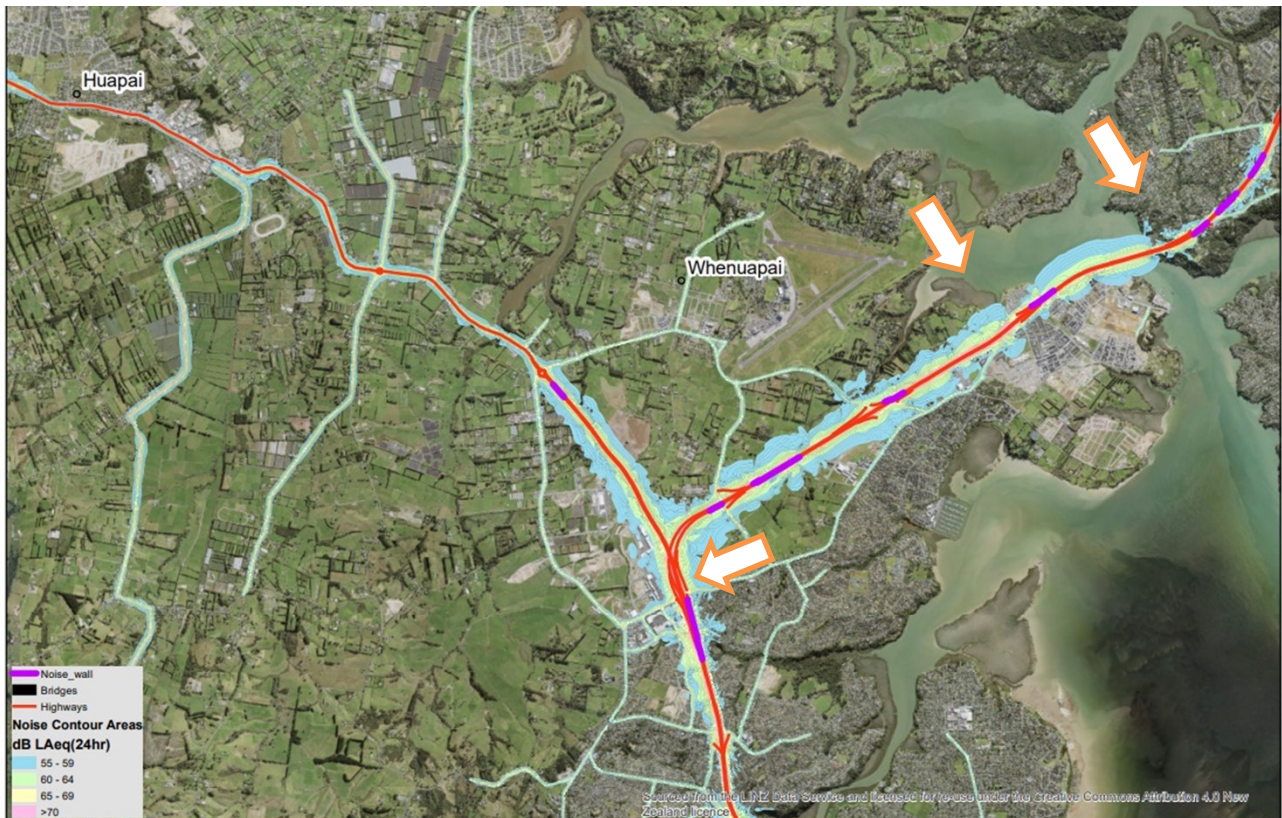
Figure 2.3 Noise walls and modelled noise contours along highways and larger feeder roads for SH16/18. The lowest noise level marked (in blue) is 55–59 dB LAeq(24). Arrows indicate where noise walls narrow the width of the 55–59 dB contour.
