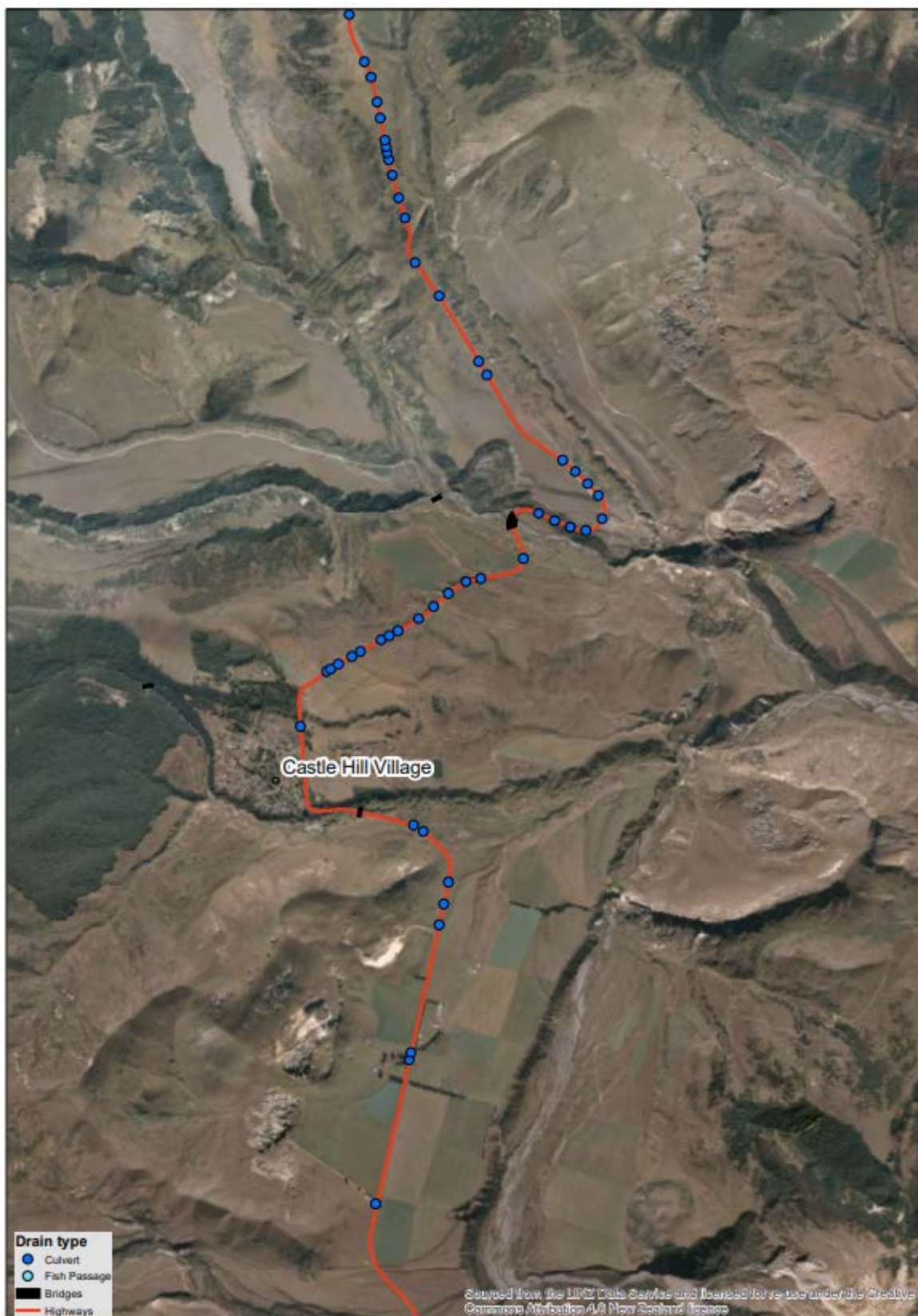
Figure 4.18 Culverts (blue dots) in the Castle Hill sub-study area. The density of culverts is influenced by slope, being low through cultivated flats and higher on steeper slopes and dissected land from Castle Hill north to Cave Stream.
