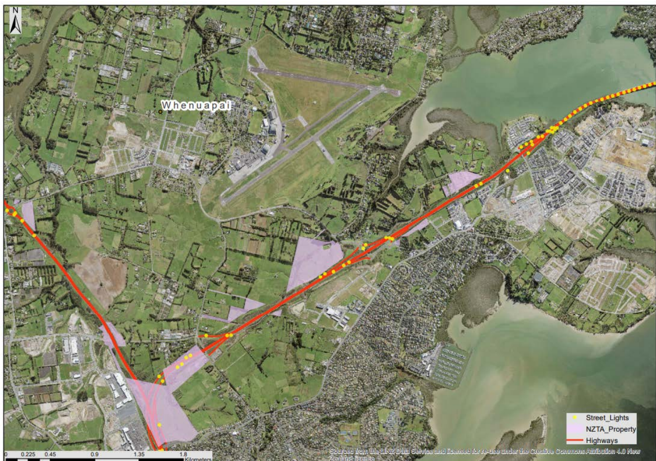
Figure 3.6 Location of streetlights and Waka Kotahi-administered Crown land in the SH16/18 case study area. Additional lighting was recorded in the field survey.
