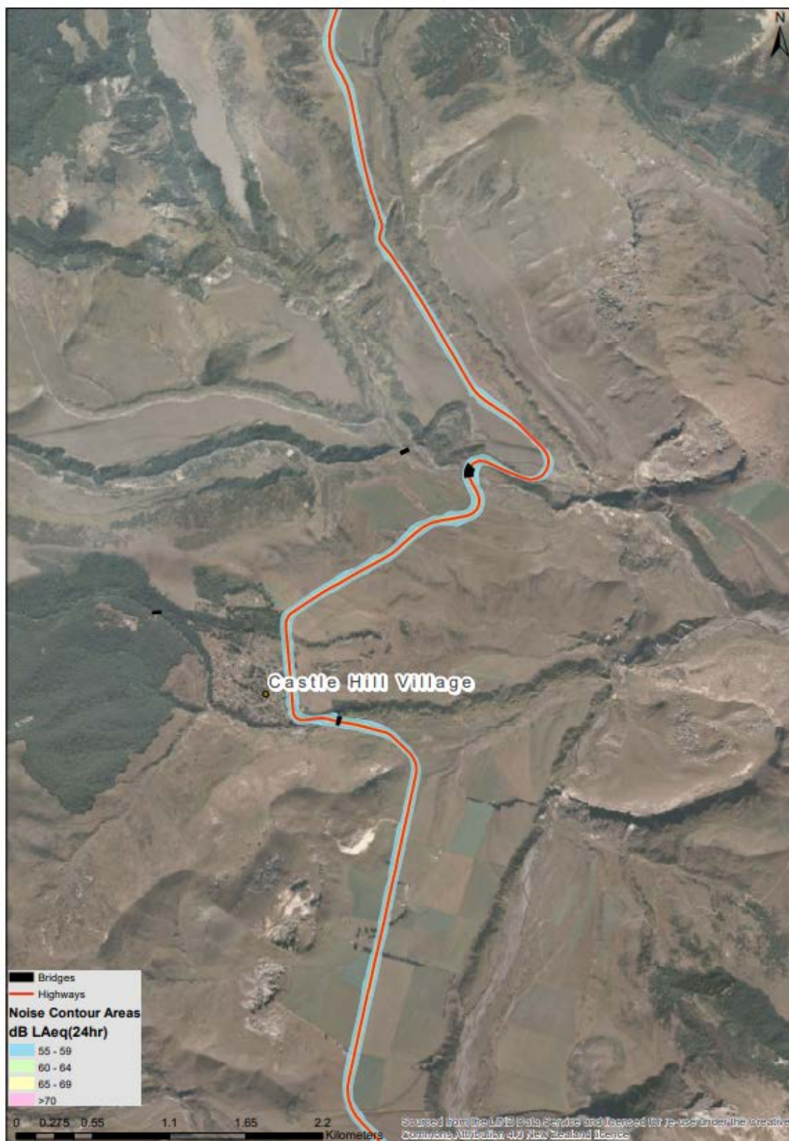
Figure 4.15 Narrow noise contours (blue) on SH73 reflect low traffic numbers and extend 25–50 m from centreline on average across the entire Castle Hill sub-study area. The northern bridge could be a site sensitive to noise and light impacts, given low background light, headlights can pass over water, and land is managed for conservation (scenic and recreational reserves).
