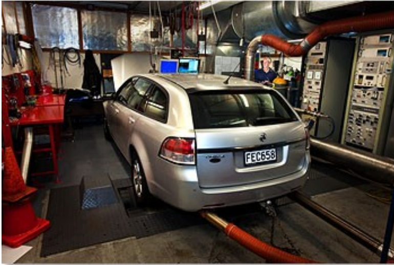
Figure 2.2 Vehicle undergoing chassis dynamometer testing at the Energy and Fuels Research Unit, University of Auckland
