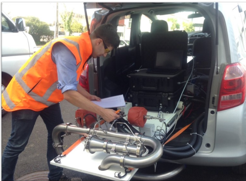
Figure 4.15 The PEMS equipment being installed in a test vehicle
