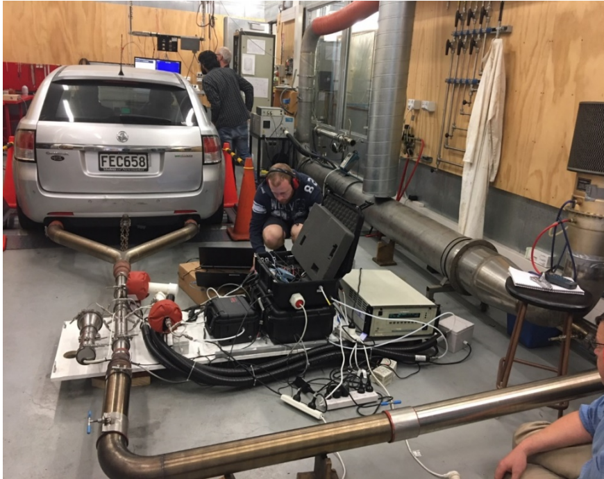
Figure 4.3 Simultaneous measurements being taken by the PEMS and the chassis dynamometer equipment
