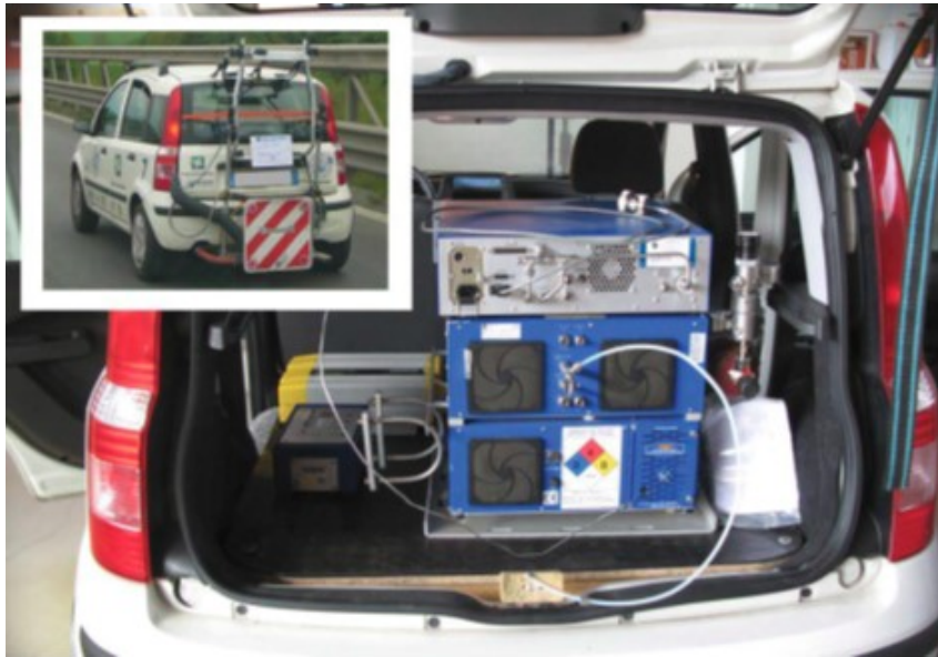
Figure 2.4 Passenger car instrumented with PEMS (Franco et al 2014)
