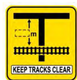
Figure L.6 Road sign indicating short stacking distance (NZ Transport Agency 2007)
