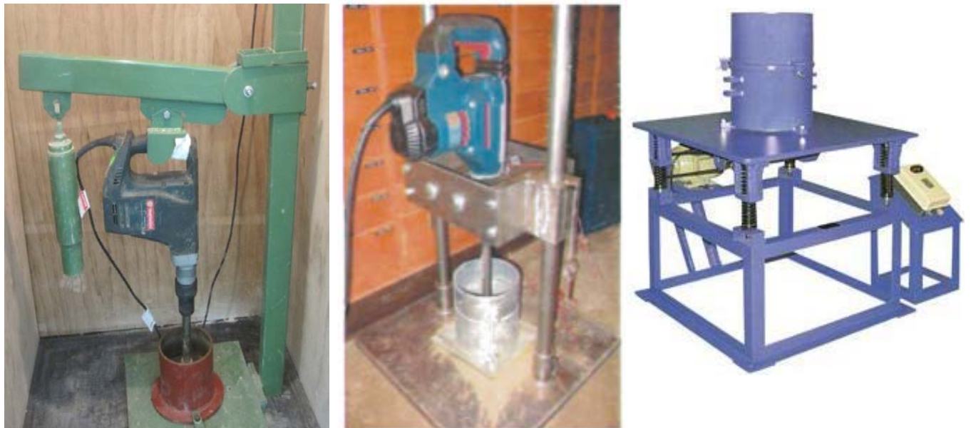
Figure 3.1 Vibrating hammer test equipment, with NZS/BSI type frame (left), ASTM type frame (centre), vibrating table (right)
